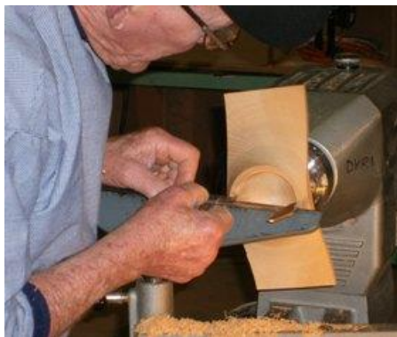
...remount using spigot, shape top, bowl, and lip for lid to fit into...
