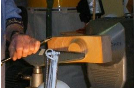
Mount using screw-chuck, shape bottom and spigot....
