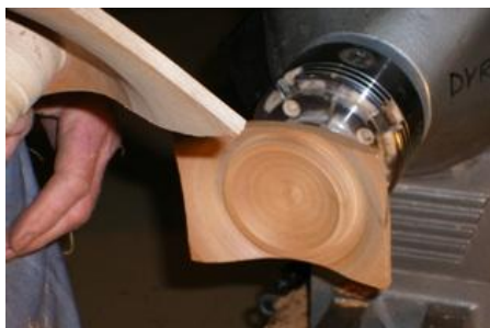
...shape underneath lid to fit base..
